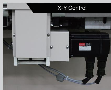
Servo motor is used for X-Y position control, allowing precise control.
