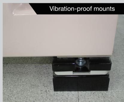
Provides anti-vibration mounts to reduce machine vibration.
