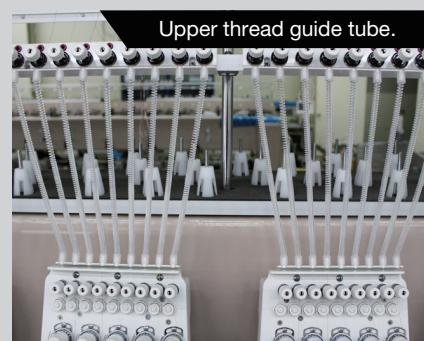
Providing the upper thread guide tube for stable supply of the upper thread.
